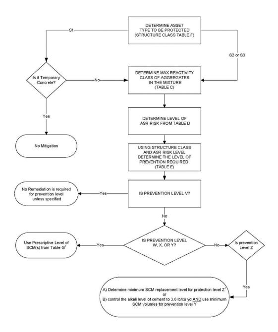
Note 1: The prevention level may be reduced by one level if low alkali cement (≤ 0.70) is used.
