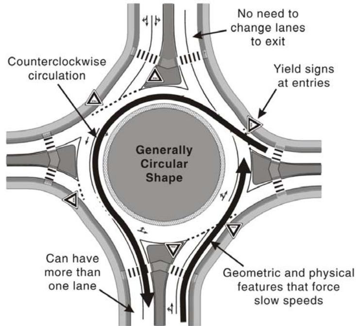
Modern roundabouts have demonstrated safety and operational benefits and should be considered as an alternative for intersection improvement projects. They can offer several advantages over signalized and stop controlled alternatives, including better overall safety performance, shorter delays, shorter queues (particularly during off-peak periods), better management of speeds, and opportunities for community enhancement or aesthetic features.
