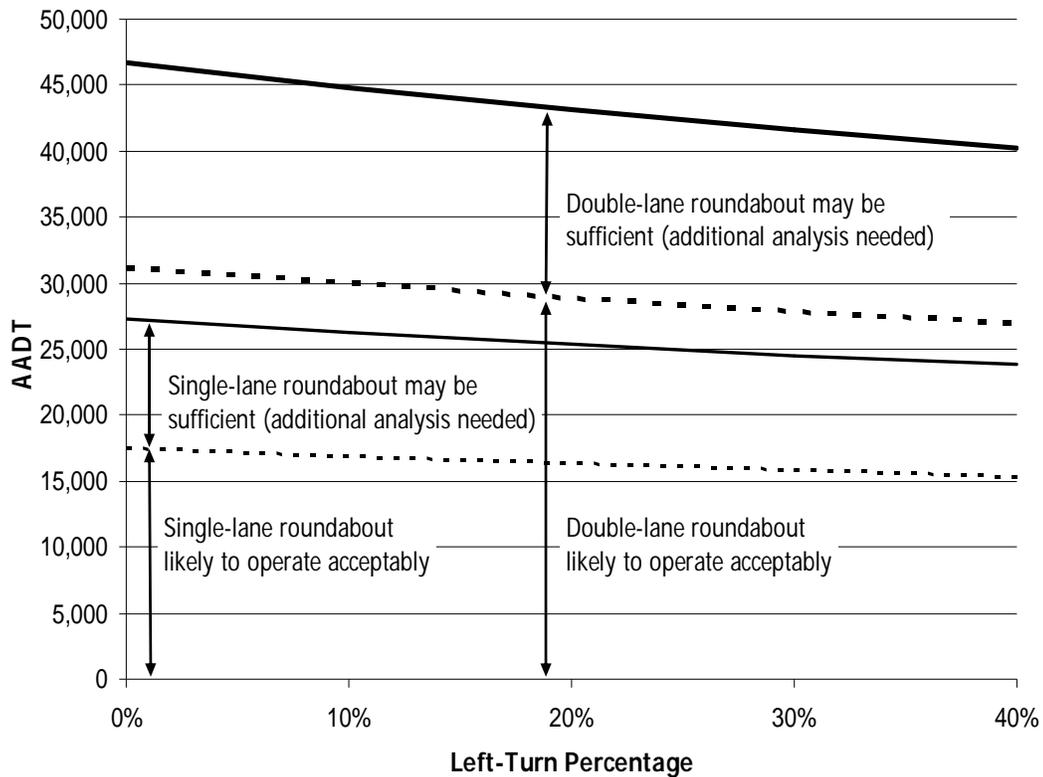
If the volumes fall within the ranges identified in Figure 3.4 where "additional analysis is needed," a single-lane or two-lane roundabout may still function quite well, but a closer look at the actual turning-movement volumes during the design hour is required. The procedure for such analysis is presented in the HCM, Chapter 21.
