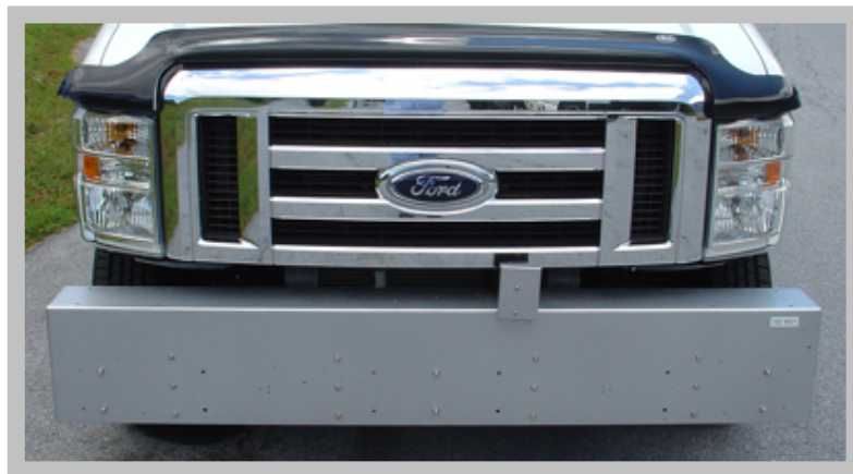
Custom Bumper containing Lasers and Accelerometers
