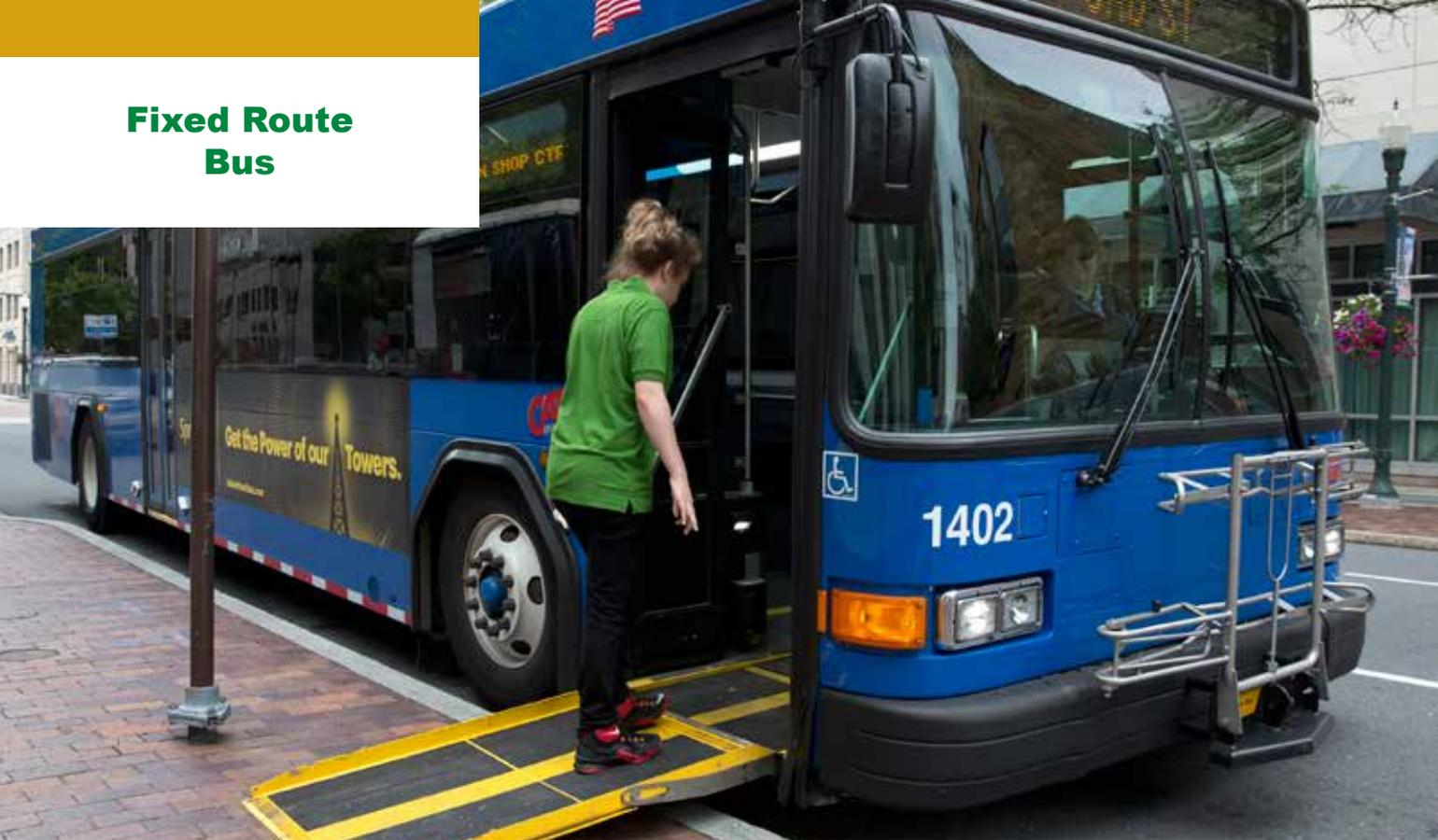
▲ Low-floor buses eliminate the obstacle of stairs. A ramp can be extended to the sidewalk.
